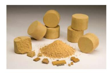
no heavy metals). Combining these new flame retardants with new resin technology and filler blends has produced a series of ultra low stress materials that resist cracking after exposure to 260°C IR reflow conditions.
